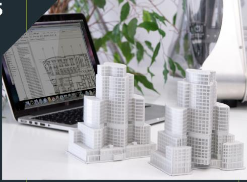
Buildings were 3D printed using Dual Extruder Toolhead. This way it was possible to manufacture the entire model in one piece even though it's built from two materials. Grey PLA was used for walls while translucent PLA imitates glass. Various 3D printing services would require you to prepare separate files to print this object in parts that you'd need to assemble later.
