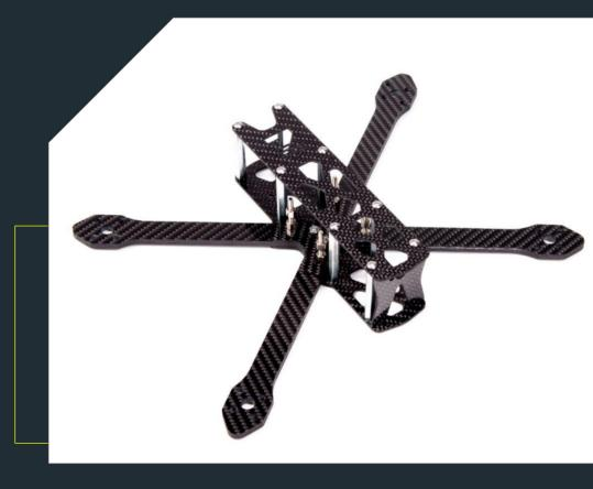
Carbon is a composite material that exhibits excellent strengthto-weight ratio and high-temperature resistance.
