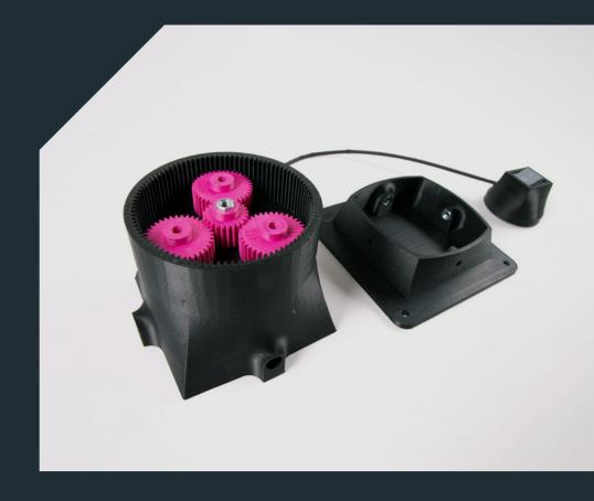
Parts used in the center planetary gear mechanism were printed with 1.75 mm ABS filaments. The standard settings were sufficient to ensure the durability of components.
