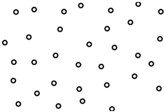
2. Place the Marker stickers on the objects' surface irregularly and ensure that there are at least 5 Marker stickers in the frame for the entire scan, or the scanner will lose track.
