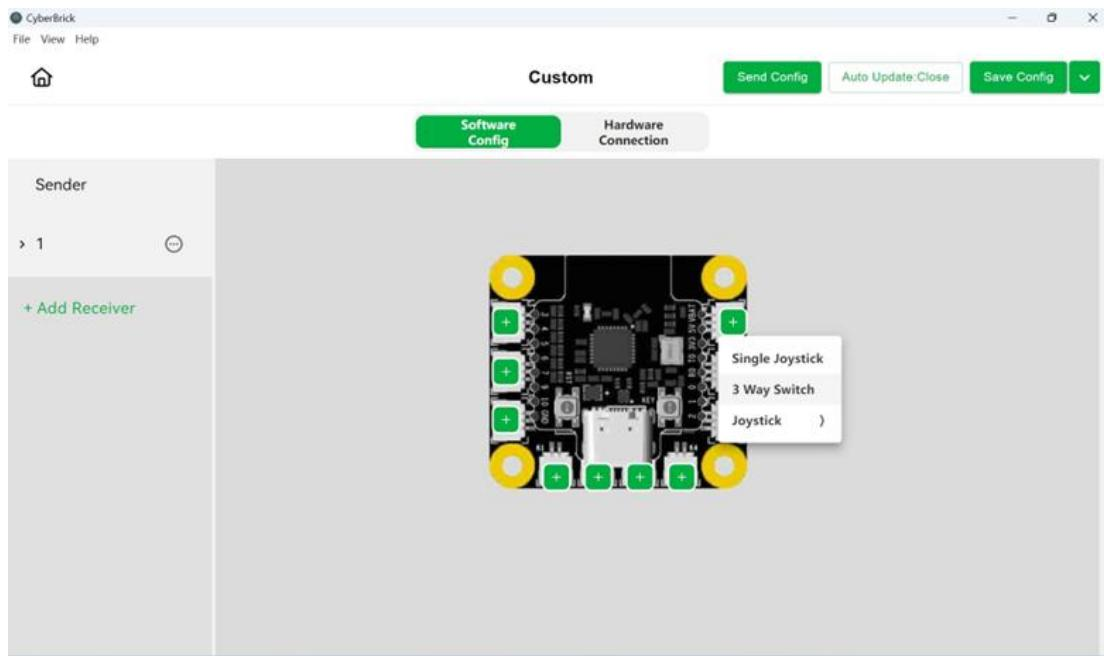
In the Modify interface of the 3 Way Switch, you can set the state of the device corresponding to the switch state, such as the light effect of the light, the speed of the motor, the position of the servo , etc. It's suitable for switching light state, controlling model deformation and other scenes.
