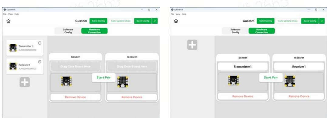
Click to start pairing. After pairing successfully, the status indicators of these devices should flash blue and yellow alternately.
