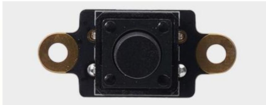
Momentary button module is a binary input module. Different signals can be sent by short press, long press, press and lift and other actions.
