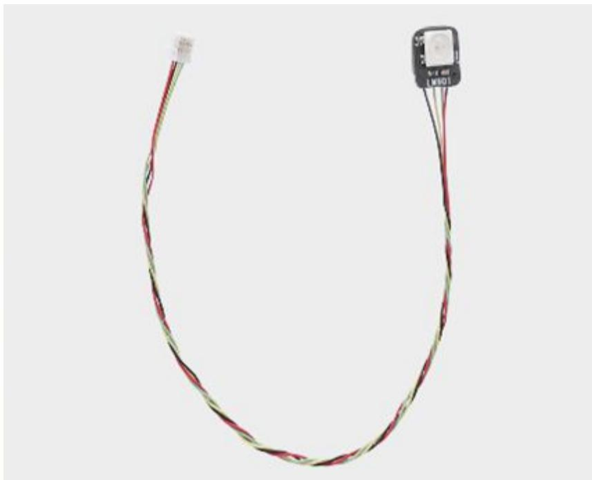
The WS2812 RGB LED is a LED board with connecting cable. It can be controlled using the WS2812 protocol and can emit multiple colors of light.
