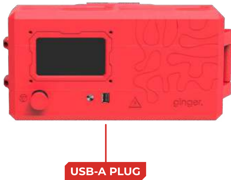
Figure 7 – Connection point for PC
